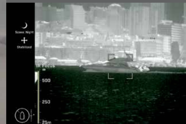
SMALL CRUISE SHIP AT DUSK VIEWED WITH THE LOW-LIGHT VIDEO CAMERA. TRACKING MODE ENGAGED TO FOLLOW THE SHIP
